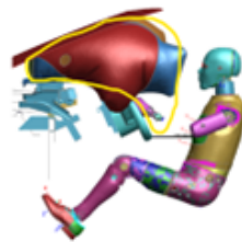
Advanced airbags for Level 3+ vehicles with foldable steering wheels
